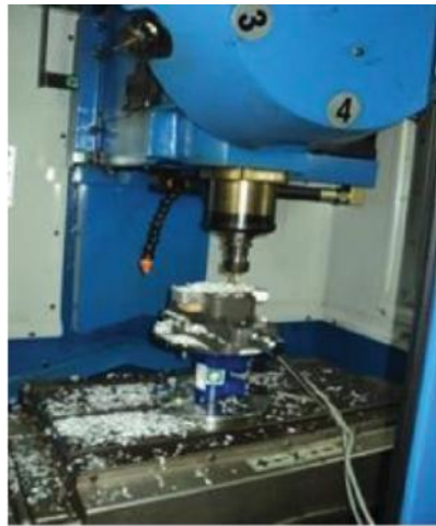
Figure 3. Arrangement used for conducting tapping experiments on composites
